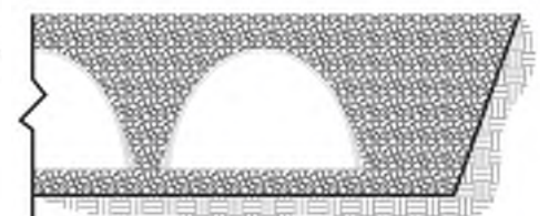
Perimeter Fully Backfilled
