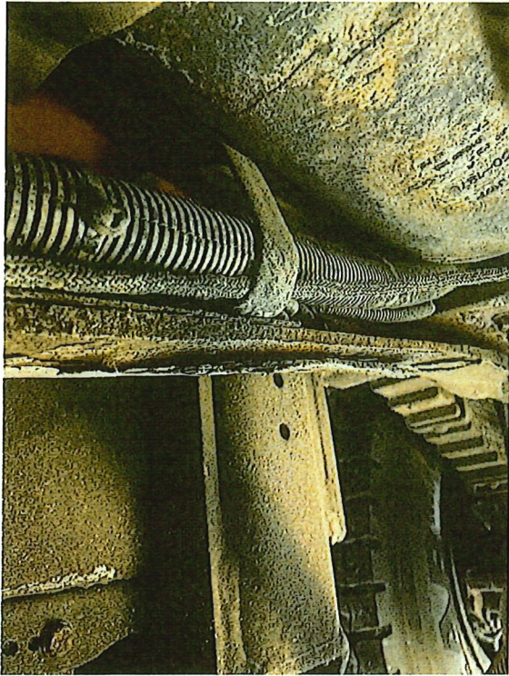
Passenger Side Inner Frame Rail Showing Delamination
