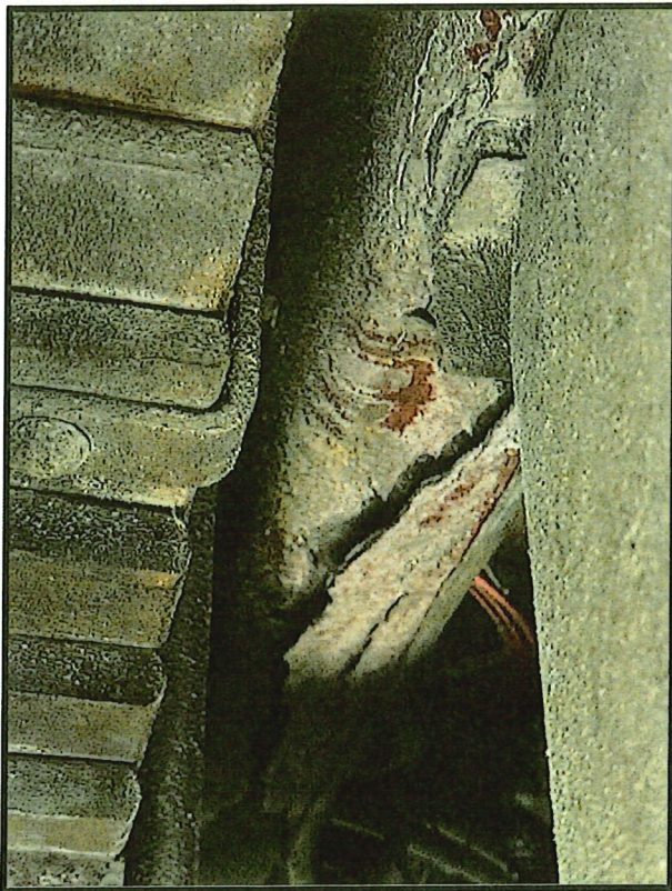
Structural Frame Rail Cracked and Delaminating
